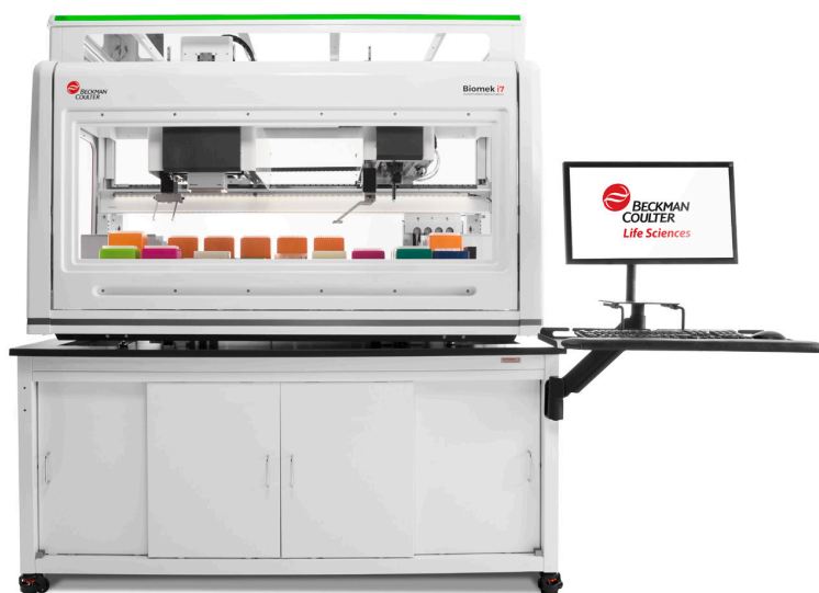
Figure 1. Biomek i7 Hybrid Automated Workstation.
