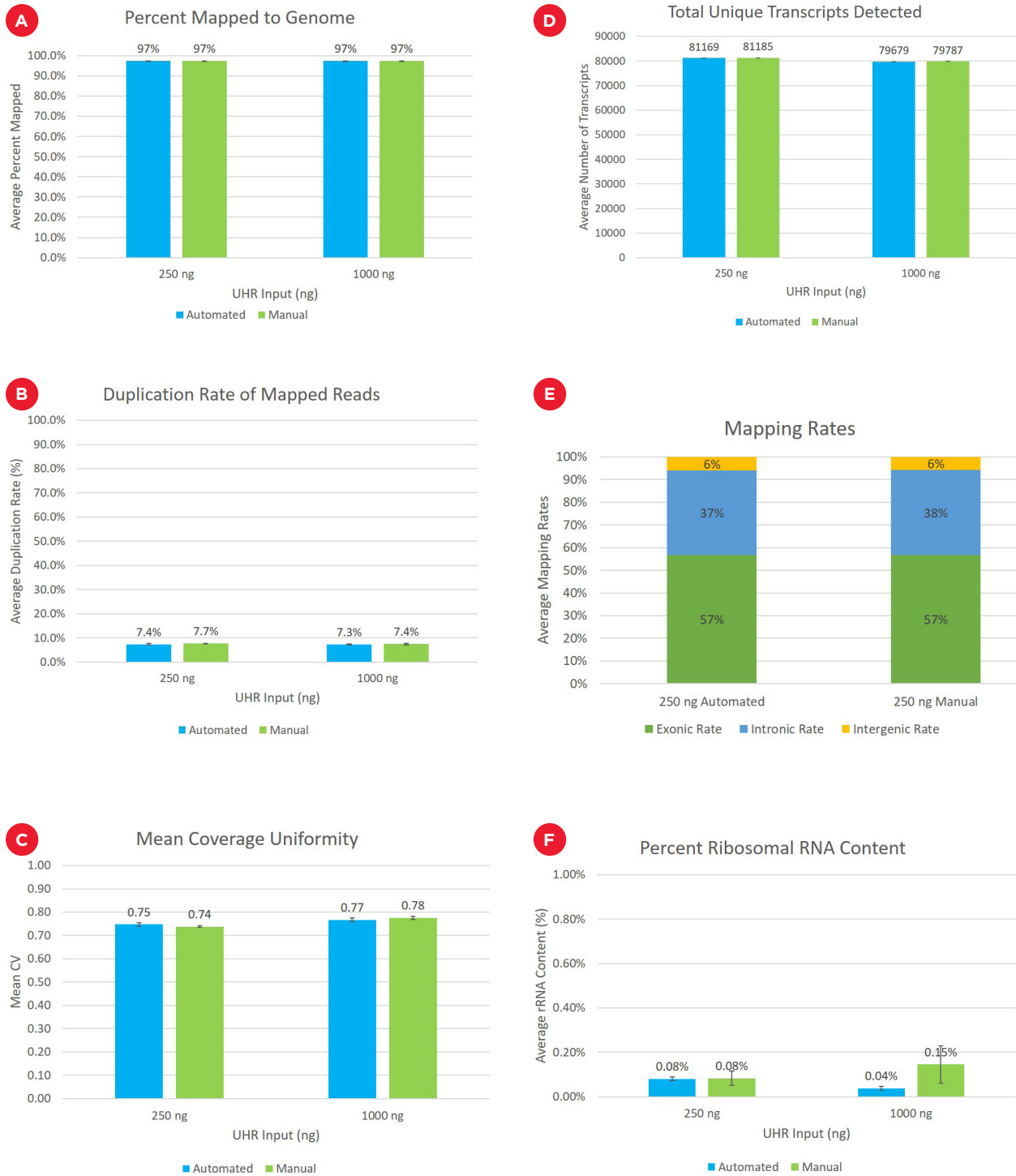
Figure 8. Comparable sequencing metrics indicate equivalent performance between automated and manual samples for both input amounts. After subsampling, data was analyzed to quantify the (a) Percent Mapped Reads (b) Percent Duplicate Reads (c) Mean Coverage Uniformity (d) Total Unique Transcripts Identified (e) Read Distribution (exonic, intronic, v. intergenic) and (f) Percent rRNA Content.
