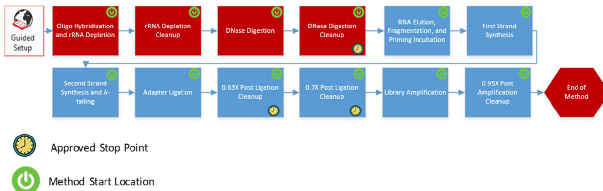
Figure 1. KAPA RNA HyperPrep Kit with RiboErase (HMR) automated method workflow on the Biomek i7 Hybrid Genomics Workstation
