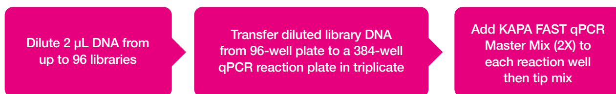
Figure 1. Overview of the steps firefly performs to automate KAPA Library Quantification Kits. The output is a 384-well qPCR reaction plate that is ready to load onto a qPCR instrument.
