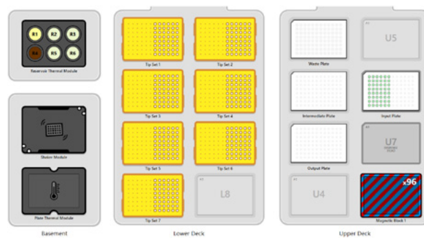
Figure 5. Starting deck layout for Optional protocol: Double-sided Size Selection. Example shown is for 6 columns of samples.
